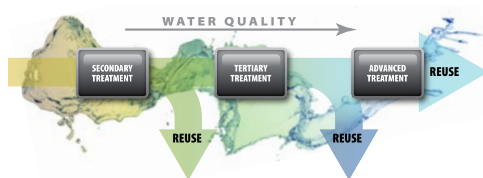
Figure 5. Water Reuse Flow Diagram Illustrates Fit-for-Purpose Quality
